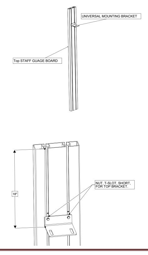
**STEP C – 1: Attach Tank Brackets**
