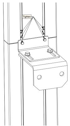
3. Attach the top Tank Bracket and mount the top Staff Gauge Board as follows. The height between the two topmost Tank Brackets is the height of the top Staff Gauge Board **minus** 13". **ALWAYS CHECK FOR LEVEL AND PLUMB**.
