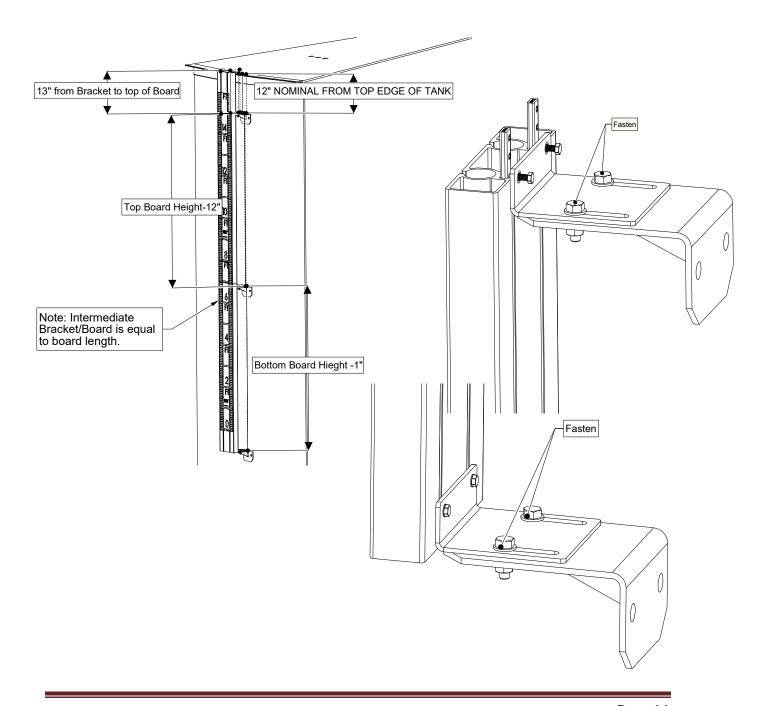
2. For each intermediate Staff Gauge Board, attach the next Tank Bracket and mount the corresponding Staff Gauge Board as follows. The height between consecutive Tank Brackets is **equal to** the height of the corresponding Staff Gauge Board. **ALWAYS CHECK FOR LEVEL AND PLUMB**.
