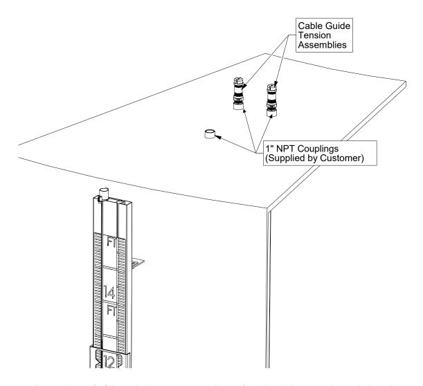
Install onto the roof of the tank the 1" NPT Coupling. If Guide Cables are to be used, then also install the two Guide Cable Tension Assemblies. The Guide Cable Tension Assemblies should be located so that the 1" NPT Coupling is at the midpoint. Refer to the diagram on the next page.
