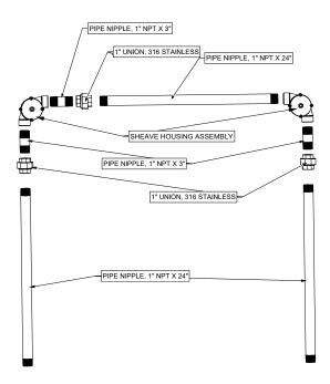
2. Pre-assemble Reeving Assembly into 4 sub-assemblies as shown .
