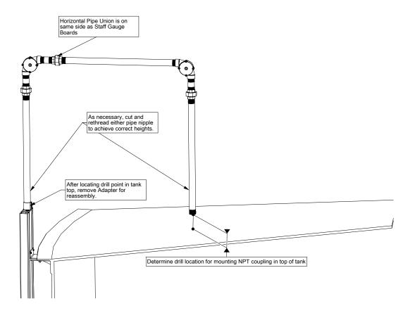
Detach the Reeving Assembly. Bring the Reeving Assembly **and Adapter** to the ground. Cut and rethread any Pipe Nipples that need to be shortened.
