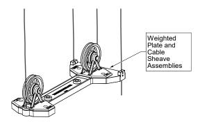
assemblies can be lowered into the tank.
