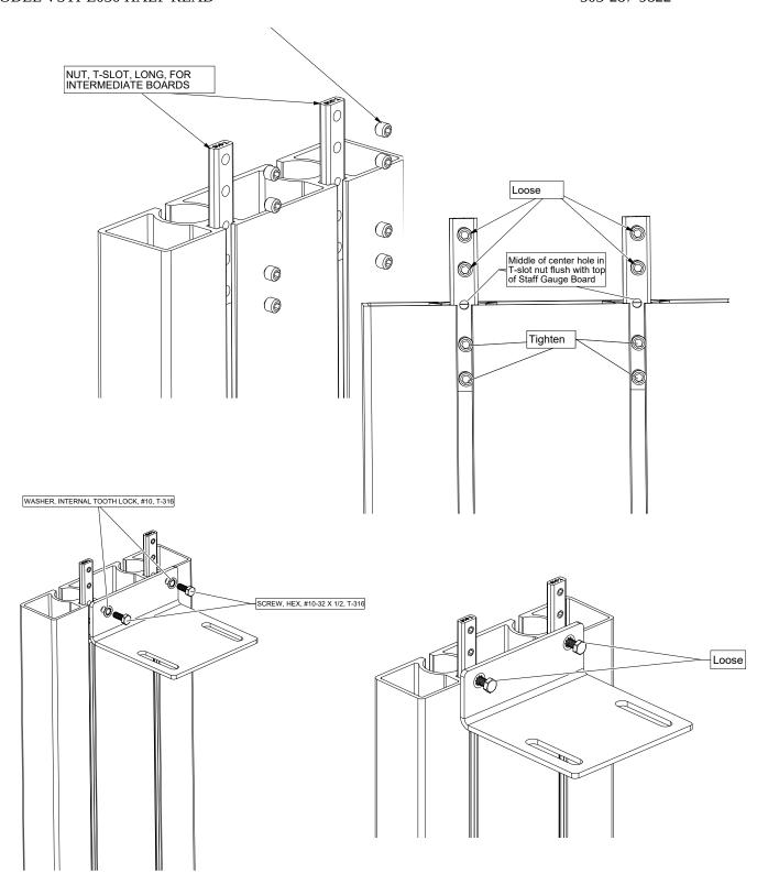
Note the 1" offset between the Universal Mounting Bracket and the top of the Staff Gauge Board. The height between Universal Mounting Brackets is therefore 1" less than the height of the bottom Staff Gauge Board. This will be important for positioning of the Tank Brackets.
