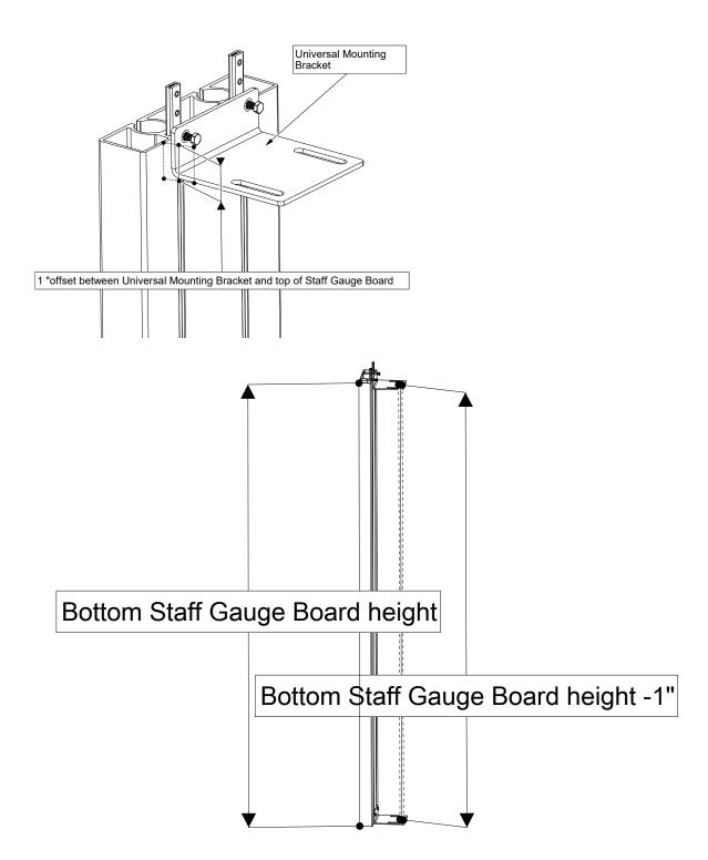
3. The intermediate Staff Gauge Boards are those in between the bottom and the top. For each intermediate Staff Gauge Board, assemble just like the bottom Staff Gauge Board but omit the bottom bracket assembly.
